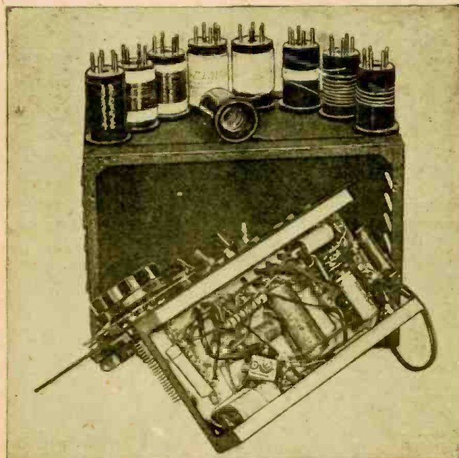
Left—Another under-chassis view, showing simplicity of wiring. Right—Top of chassis and inside of panel. The three controls are for intensity of oscillation, pitch of audio modulation and strength of output.
